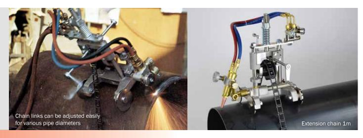
The Picle-1 is a manually operated pipe cutting machine for cutting and bevelling pipes. Equipped with a chain and worm gear drive system with low transmission ratio, leading to an absolutely frictionless feel.
